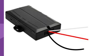
**RED**= Permanent Power (Must be fitted with Max 5A fuse in line)
